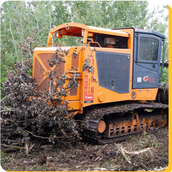
Our forestry crews use equipment like this mulcher to clear vegetation along power lines and help prevent wildfires.
