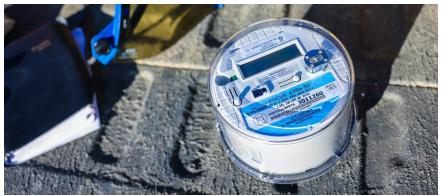
The electrical meter on your home, farm or business is equipped with a proven technology that enables FortisAlberta to read it remotely instead of physically coming onto your property to read it. Your meter is wired to and sends reads containing your total electricity consumption directly through the existing power lines once per day.
