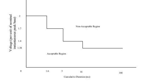
The DER shall not contribute to instantaneous or fundamental frequency overvoltages with the following limits:
