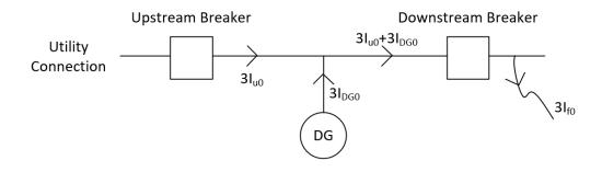
The de-sensitization of concern is the fault flow currents designated  $3I_{u0}$  in the diagram above.
