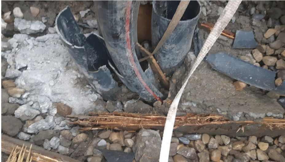
Figure C3.1 Ducting damaged while pulling cable.
